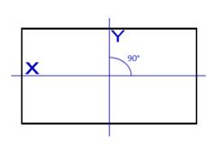
5. A herringbone design should typically be started from a central axis, using a chalk line or straight edge to mark the centre of your room create the 'x' line, then a second line needs to intersect this line at 90° to create the 'y' line. Setting this axis up is crucial and its good practice to check all angles and measurements are correct at this stage before any planks are laid.
