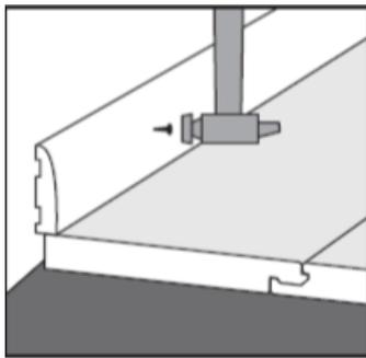
The expansion gap can be covered with a trim or a skirting suitable enough to cover the gap. These should be fixed to the wall, never to the flooring.
