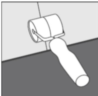
Using an off cut of the product with a rubber mallet is recommended for assisting in fitting the boards, a hand roller can help secure the boards over the joints.
