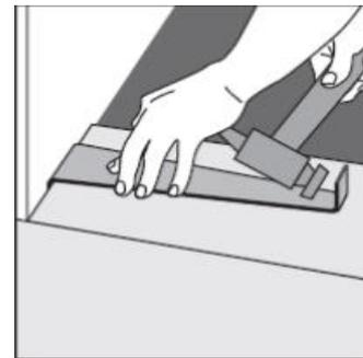
The remainder of the row is completed using these techniques. A pull bar can be used to pull the boards together around the edges of the room. Repeat this method until your installation is complete.
