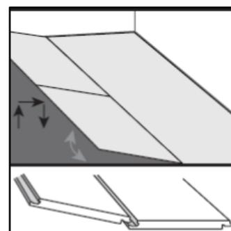
The 2nd row is started by clicking in the tongue of the 2nd row starter board into the groove of the board on the first row at approx 30° the board is fixed by pushing it firmly in the first row.
