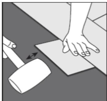
Fit the next board by clicking the tongue and groove together along the short edge. Ease the tongue and groove together along the long side by angling the boards together.
