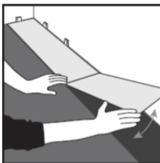
The first row is laid by clicking the end joints together, cut the last board in the row to size making sure the 5mm expansion gap has been left.
