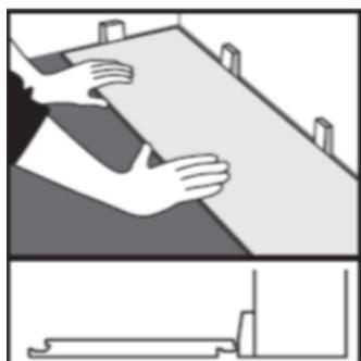
Install the first plank or tile with the longer tongue side of the board facing the wall, use spacers to give a 5mm expansion gap between the board and the wall.
