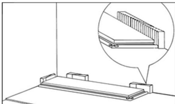
Starting from the longest straight wall of the room, the first board is laid with the short edge or Tongues edge facing the wall and the Longer edge or Groove edge facing the installer.
