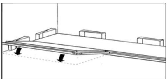
To start the second row place the short edge side of the starter board into the groove of the long edge side of the previous fitted row at a slight angle, a tapping block can be used to help fully locate the new board if required, it can now be lowered to the floor to complete the joint between rows.
