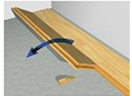
3. Start the next row with the piece left over from the previous row. It must be at least 50cm long, if the piece is too short start with a new board cut in half. Always ensure the end joints are staggered at least 50cm.
