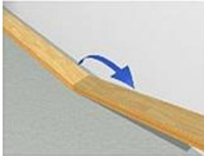
2. Press the next floorboard at an angle to the first one and lay it down, complete the first row in the same way, cut the last board to start the next row.
