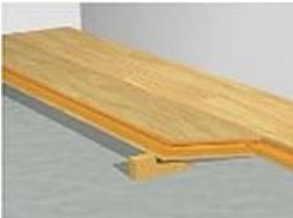
4. Place the floorboard at an angle against the first floorboard in the previous row, push forwards and press down at the same time, place a wedge under the board.
