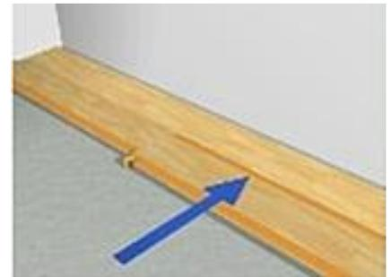
6. Use a hard striking block to close the long side joint, do not force the boards together move out the wedge and place it under the next board.
