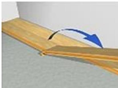
5. Press the next floorboard at an angle to the previous one and lay it down to the same level.
