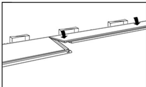
Expansion must be allowed between the wall and the board using spacers from an installation kit a minimum gap of 10mm is recommended however for larger rooms this may need to be increased. To connect the second board to the first place the interlocking end of the second board at an angle to that of the already installed board and then lower to the floor to complete the joint, continue this to build up the first row in this way.
