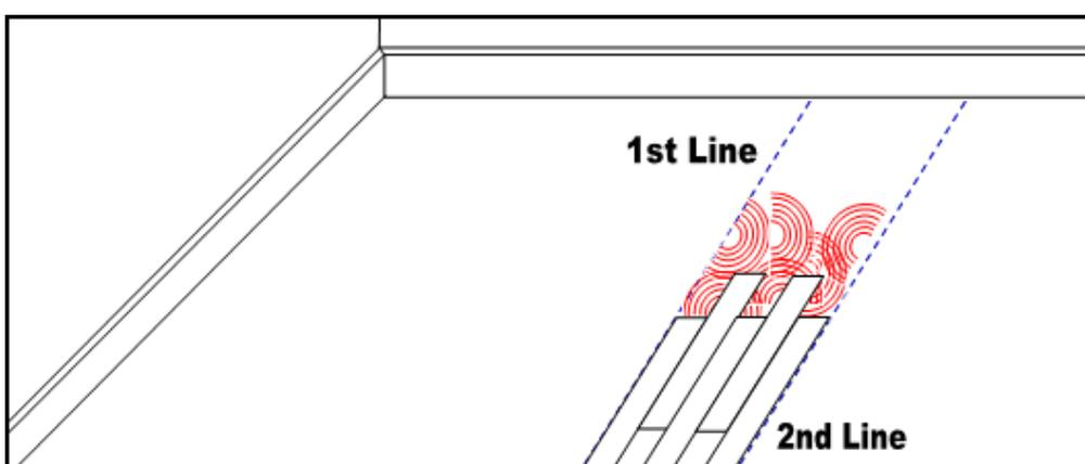
3. Spread the adhesive evenly across the area until it reaches its optimum bonding strength, Planks or tiles can then be laid into the adhesive, remember to observe the direction arrows printed on the underside of the plank or tile.
