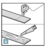
Some boards will require cutting, observe the cutting direction of the blade to prevent breakout, handsaw's cut from the décor side, jigsaws with an upcutting blade cut from the rear of the board.
