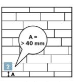
Measure the length and width of the room to plan a balanced appearance. If the last row is less than 40mm it will be easier to cut down the first row to give balance between the two rows.
