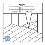
As the floors will expand and shrink depending on the current climate it is vital that the 8-10mm gap is maintained around all obstacles including door frames, pipes and around all edges of the floor.
