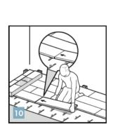
As your installation grows, place a full pack across the installed rows, flip your position onto the installed side and connect the short end of the panel.
