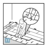
The boards can be clicked together by placing both hands close to the joint and pulling towards you on the long side.
