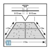
If the length or width of the room exceeds 13m further expansion will need to be added to accommodate the floor as it expands and shrinks.
