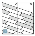
Always work out of more than one box to allow for a good mixture of colours and tones. It gives a good visual effect if the floor boards are fitted in the same direction as the longest wall and parallel to the incidence of light.
