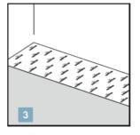
Install the underlay as per width and add a new layer as the installation continues. Underlays will help smooth unevenness, insulate, reduce noise. Quick Step offer a full range including underlays with a vapour barrier.
