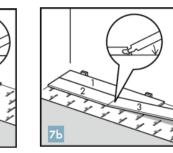
To install a panel, position it at an angle of 20° to 30° to the panel already fitted. With a gentle rocking motion up and down and applying forwards pressure the panels will click into place automatically.
