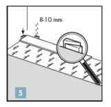
Use spacers between the planks and the wall, this will ensure that your expansion joint is wide enough and maintained between 8 – 10mm.
