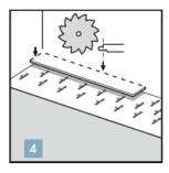
Begin the first row with a full plank, with a saw cut off the tongue from the long and short side, these will be placed next to the wall.
