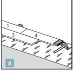
Uniclic also allows you to tap the panels into each other without the lifting, a Uniclic tapping block must be used, take several taps to join <u>never</u> a single blow.
