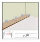
Mark the last panel in the first row to the required length (place tongue to tongue) and cut. Start the second row with the off cut from the last panel of the first row. Always make sure the off cut is at least 200 mm (8") long, if not then cut another piece which is greater than 200mm long. Start all subsequent rows with the off cut piece from the previous row.
