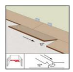
The second panel is located in the groove of the first row in the same way, once located the second panel can be slid towards the first panel of this row, when they meet the new panel can be lowered to the sub floor to lock it into position, apply pressure to the head joint to complete the joint
