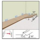
The second row is started by using the off cut from the previous row if it's greater than 200mm, at an angle place the tongue edge to the groove edge of the first row, don't forget to allow for expansion at the beginning of the second row, once located the new panel of the second row can be lowered to the sub floor locking the newly formed joint.
